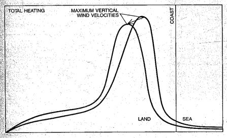
TOTAL HEATING of a column of air over the land is the sum of three contributions: radiative heating (not shown), sensible heating (from the sun-warmed land) and latent heating (from the condensation of water vapor). Precipitation tends to reduce the sensible heating of the column, causing the maximum total heating to shift inland. The region where the ascending air has its maximum velocity also shifts inland and a slow migration of the active monsoon ensues.
